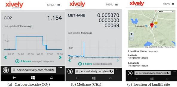
Figure 11.Screen shots of Uploaded gas concentrations and location of landfill site on a web page.
