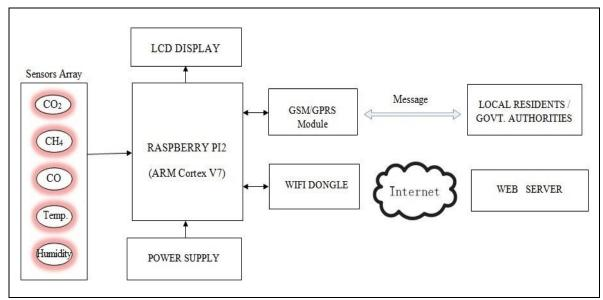
Figure 3. Block diagram of remote environmental monitoring system.
